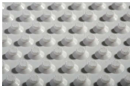
A belt-conveyor provided with nozzles
